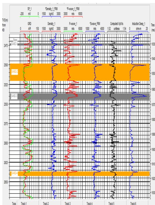
Gambar 4. Log data of #L-30 well containing oil saturated sandstone from Middle Missisauga formation
